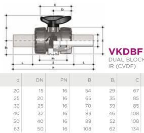
DUAL BLOCK<sup>®</sup> 2-way ball valve with long spigot male ends in PVDF for butt welding/ IR (CVDF)
